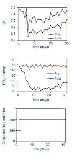
Figure 2: Circulation pump rate, pH and  $PO_2$  from one 160-mL bioreactor.
