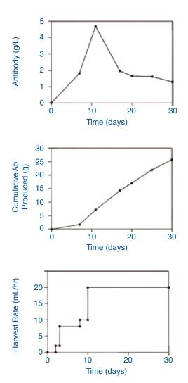
Figure 3: Antibody concentration, cumulative antibody production, and harvest rate from one 160-mL bioreactor
