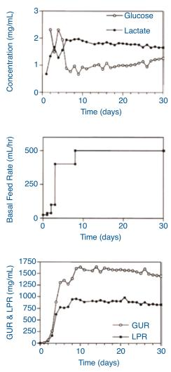
Figure 1: Basal medium feed rate and glucose and lactate metabolism from one 160-mL bioreactor.
