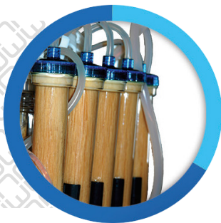
Photo showing five of the ten bioreactors during a production-scale run in AcuSyst-XCELLERATOR ™
